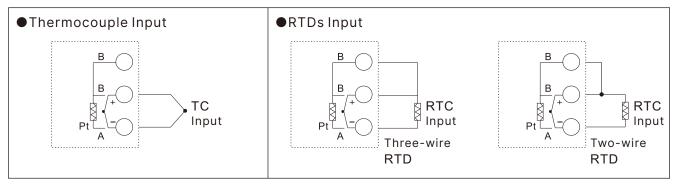
\*If the input wiring is incorrect or the sensor is damaged or out of range or the Int setting is inconsistent with the input sensor type, the second display window will display a "orAL" warning flashing. After you eliminate these faults, the instrument will display the measured values normally.
